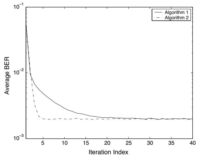
Fig. 3.  $K = 4$  user MIMO system with  $M_i = 1$  data streams per user.  $N_{T_i} = N_R = 4$ . BER analysis at each iteration.
