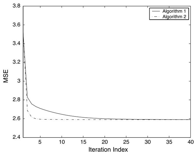
Fig. 7.  $K = 3$  user MIMO system with  $M_i = 2$  data streams per user.  $N_{T_i} = 4$ ,  $N_R = 4$ .
