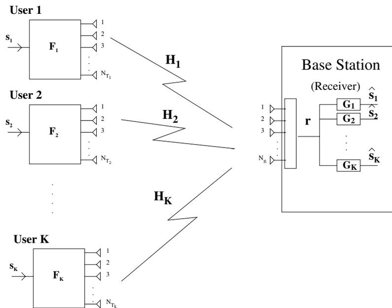
Fig. 1. System model of multiuser MIMO system.
