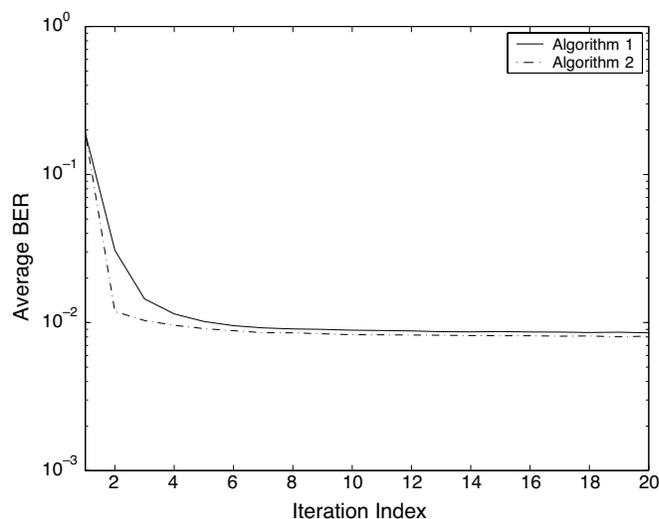
Fig. 6.  $K = 2$  user MIMO system with  $M_i = 2$  data streams per user.  $N_{T_i} = 4$ ,  $N_R = 4$  BER analysis at each iteration.
