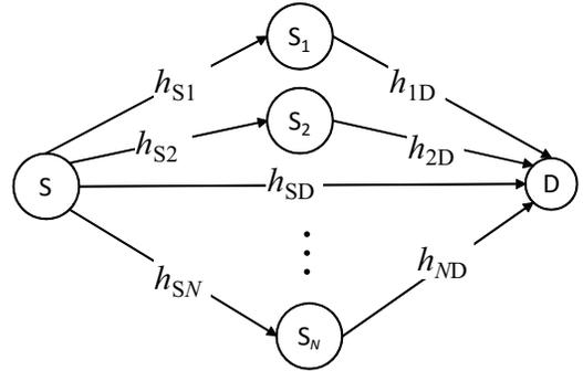
Figure 5. System model with  $N$  potential relays.
