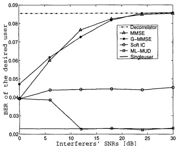
**Figure 1.** Coherent detection for BPSK. Desired user at 6 dB SNR.  $N = 7$ ,  $K = 4$ , Gold sequences.
