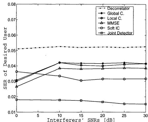
**Figure 2.** Noncoherent detection for nonlinear modulation. Desired user at 10 dB SNR.  $N = 20$ ,  $K = 2$ ,  $M = 4$ , random sequences.
